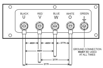
Figure 27. Output Terminal Lugs 3Ø-480/277V Connections
